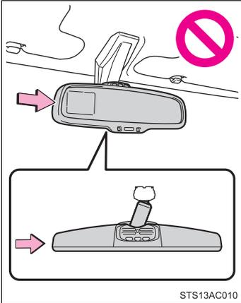
Do not push the mirror horizontally from the side. The mirror could fall off.
