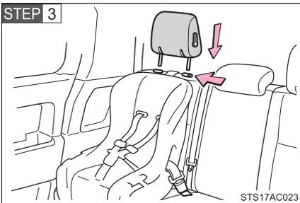
Reinstall the head restraint.
