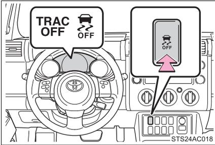
Press and hold the switch for more than 3 seconds while the vehicle is stopped to turn off TRAC and VSC.
