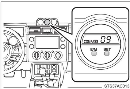
**STEP 2** Press the SET button until a number (1 to 15) appears on the outside temperature display.
