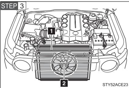
After the engine has cooled down sufficiently, inspect the hoses and radiator core (radiator) for any leaks.
