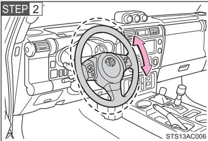
Adjust to the ideal position by moving the steering wheel vertically.
