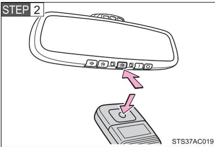
Press and hold down one of the buttons on the HomeLink® and the button on the transmitter. When the indicator on the HomeLink® changes from a slow to a rapid flash, you can release both buttons.
