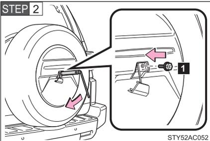
Install the spare wheel cover in the reverse order of removal.
