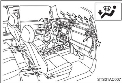
When the dial is set to
