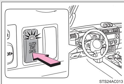
Press the CLUTCH START CANCEL switch to cancel the clutch start system with the engine switch is turned to the ON position.
