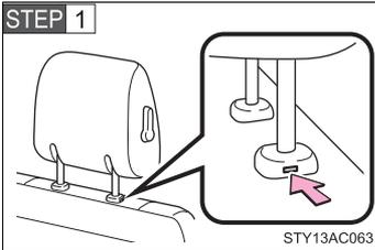
Push a flathead screwdriver into the slot. The slot is located on the right side of the right head restraint anchor.
