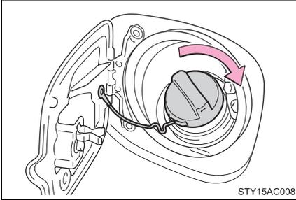
When installing the fuel tank cap, turn it until you hear a click.
