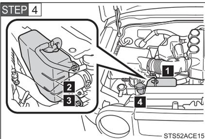
The coolant level is satisfactory if it is between the F (Full) and L (Low) lines on the reservoir.
