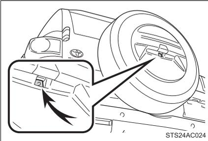
The camera for the rear view monitor system is located to the spare wheel cover.
