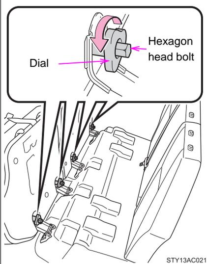
Loosen the bolts with a wrench at first and turn the dials by hand to remove them.
