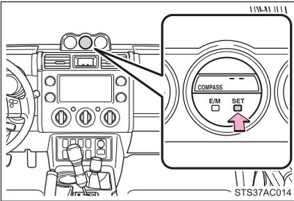
**STEP 2** Press the SET button until the zone number appears on the outside temperature display.
