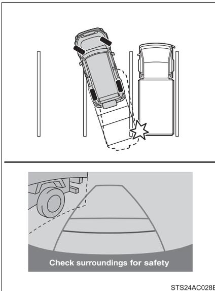
Visually check the surroundings and the area behind the vehicle. In the case shown in the illustration, the truck appears to be outside of the vehicle width extension guide lines and the vehicle does not look as if it hits the truck. However, the rear body of the truck may actually cross over the vehicle width extension guide lines. In reality if you back up as guided by the vehicle width extension guide lines, the vehicle may hit the truck.
