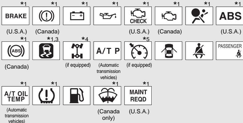
\*1: These lights turn on when the engine switch is turned to the ON position to indicate that a system check is being performed. They will turn off after the engine is started, or after a few seconds. There may be a malfunction in a system if a light does not come on, or if the lights do not turn off. Have the vehicle inspected by your Toyota dealer.
