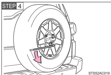
Turn the hold-down nuts counter-clockwise with the wheel nut wrench and remove them.
