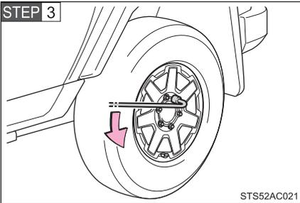
Slightly loosen the wheel nuts (one turn).
