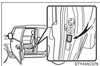
For the GAWR, see the Certification Label. For the maximum load of the tire, see the load limit at maximum cold tire inflation pressure mentioned on the sidewall of the tire. (→P. 526)
