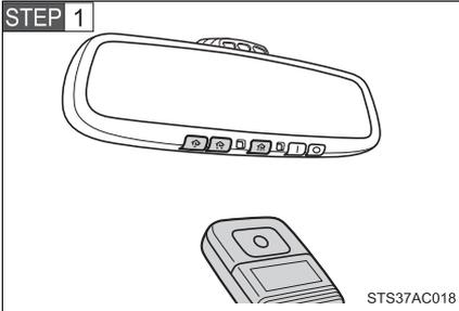
Point the remote control transmitter for the device 1 to 3 in. (25 to 75 mm) from the HomeLink® control buttons.
