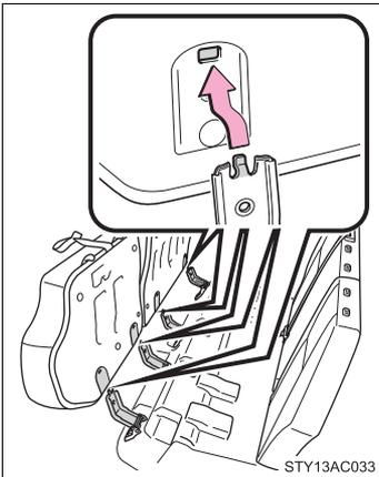
Click the claw of the hinge into the hole of the bottom cushion before refastening the dial.
