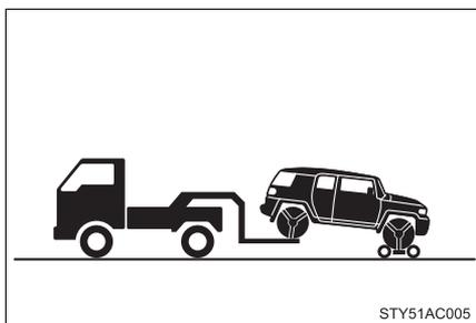
Vehicles with an automatic transmission: When not using a towing dolly, turn the engine switch to the ACC position, shift the shift lever to N and shift the front-wheel drive control lever in H2.
