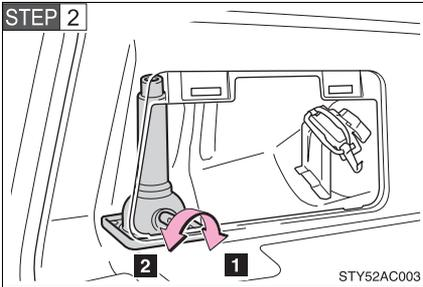
Loosen and remove the jack.
