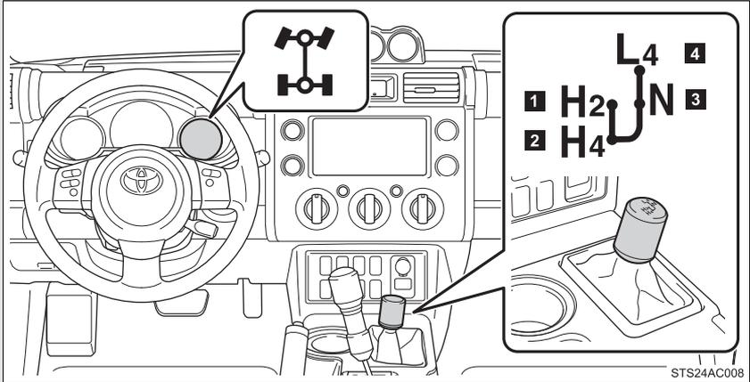
The four-wheel drive indicator comes on when the H4, N or L4 mode is selected.
