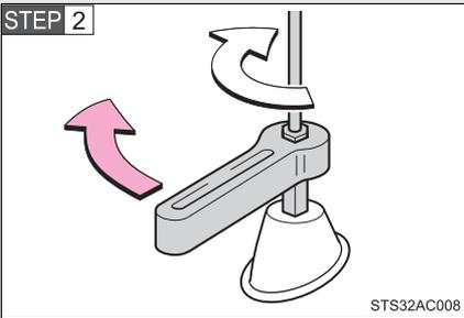
Using the wrench, tighten the antenna an additional 1/8th turn (20 to 45 degrees) to secure it in place.
