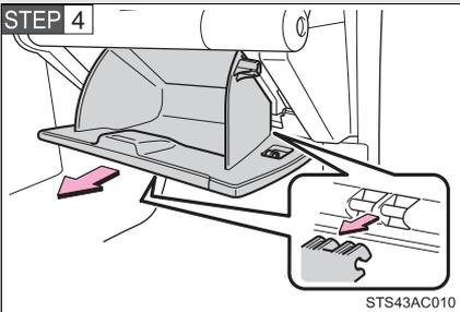
Then disconnect the claws at the bottom and remove the glove box.
