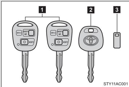
**1** Master keys (with wireless remote control function)
