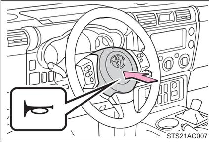
To sound the horn, press on or close to the
