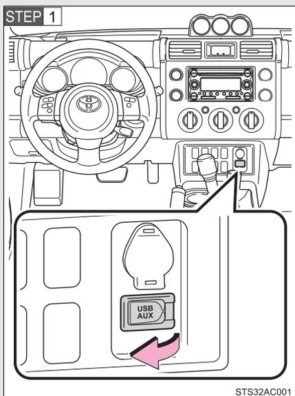
Open the cover and connect the portable audio device.
