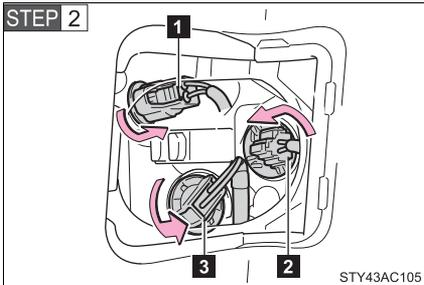
Turn the bulb bases counter-clockwise.
