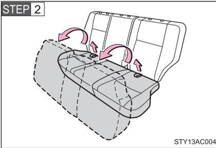
Swing the bottom cushion up by pulling the lock release strap.
