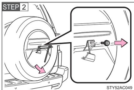
Remove the bolt which fixes the spare wheel cover using the wrench in the tool bag (→P. 484).
