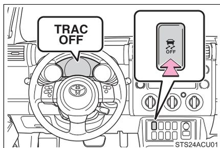
Quickly press and release the switch to turn off TRAC.
