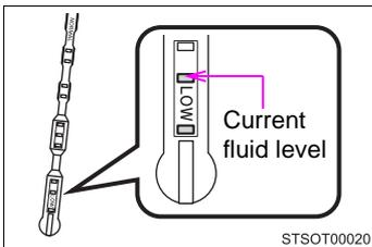
The washer fluid level can be checked by observing the position of the level on the liquid-covered holes in the gauge. If the level falls below the second hole from the bottom (the LOW position), refill the washer fluid.
