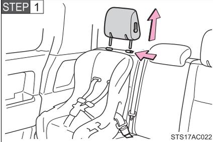
Secure the child restraint using the LATCH anchors or seat belt, and remove the head restraint.
