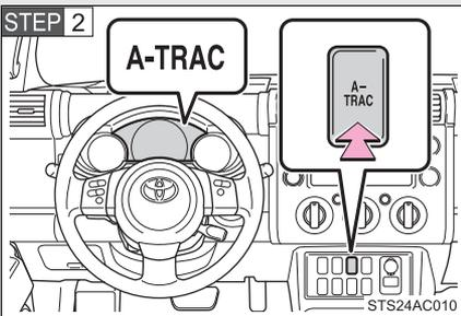
Press the A-TRAC switch to activate the system.
