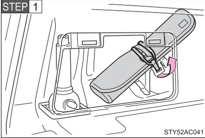
Remove the cover and loosen the strap.
