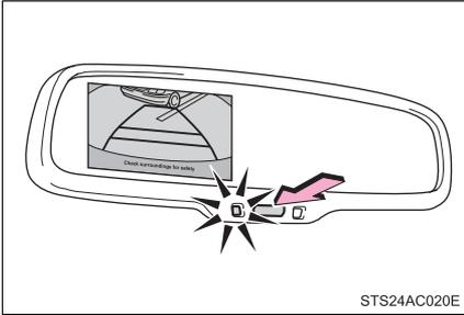
When the screen is displayed, press **AUTO** on the inside rear view mirror to switch the screen ON/OFF mode.
