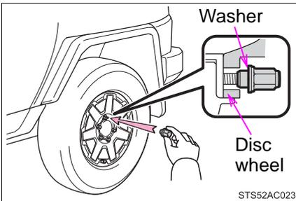
Tighten the nuts until the washer of the nut comes into loose contact with the disc wheel.
