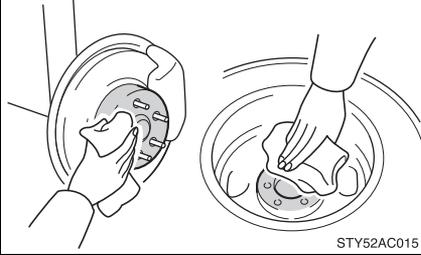
Remove any dirt or foreign matter from the wheel contact surface.
