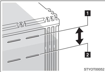
Check that the level is between the upper line and the lower line.
