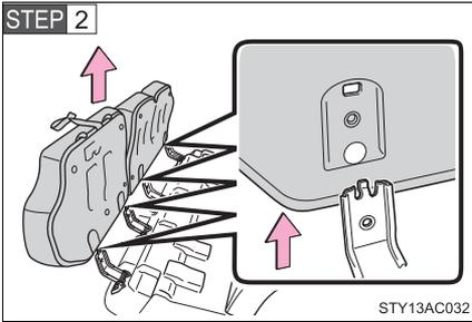
Separate the bottom cushion from the hinge.
