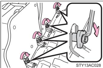
Firmly tighten the hexagon head bolts using a torque wrench.
