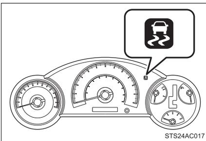
If any of the drive wheels spins, the slip indicator flashes to indicate that the active traction control system have been engaged.
