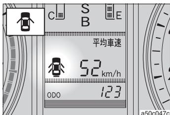
"Engine start stop" switch is also at . ON " (smart entry & start system non-installation car) ignition ON mode (smart entry & start system installation car) or the engine switch to lighting a half door warning light ( P. 263) and is displayed.
