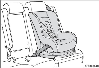
Seat belt with child seat fixation mechanism
